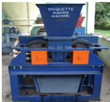
Charcoal Briquetting machines at RARS, Chintapalle
