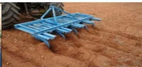
Tractor drawn 9 - tyne (spring) cultivator
