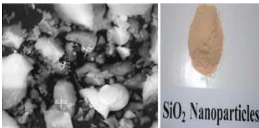
Scanning Electron Microscopic image of nanoscale silicon dioxide
