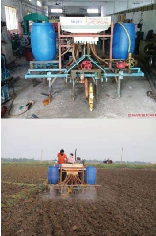
Fig: Planter cum herbicide applicator working in field
