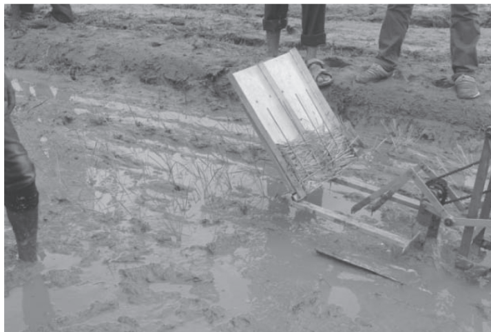
Fig. 8. Developed 2-row manually operated rice transplanter during operation
